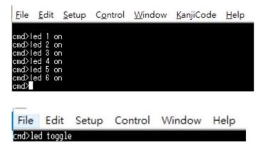
There are two Tri-color LEDs on location LED2 and LED3 built in board. Parameter LED1 is **Green**, LED2 is **Red**, LED3 is **blue** color in LED2 Parameter LED4 is **Green**, LED5 is **Red**, LED6 is **blue** color in LED3
